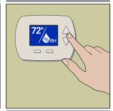
**Maintain** Environment Interior temperature should be maintained between 65° and 85°F during the service life of the floor.
