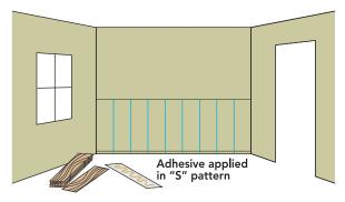
• Set plank in place with the top of the plank on the chalk line leaving a minimum 1/2" expansion space at bottom of wall.
