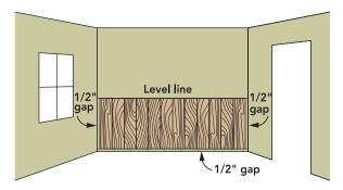
Trim out walls using 3/4" round (avoid nailing into planks). Install baseboard to cover gap along floor and Install threshold along top edge to finish wainscot wall.
