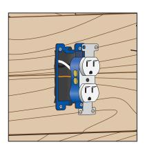
Do not cover receptacle retaining screw /surrounding fixture, to allow for bringing receptacle forward to accommodate for the thickness of new planks.
