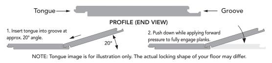
Cut off the tongues on the first row of planks. Be sure locking system is fully engaged! Planks must be flat in relation to each other (on all sides) without gaps before continuing installation.
