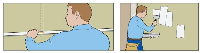
• Make repairs and remove any loose paint, wallpaper and all other contaminates that may affect adhesive bond (prime & paint repaired areas).
