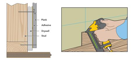
Use a level to double-check the levelness of the line between the two marks. Adjust line as needed with spacers. Secure this first row fully using adhesive and 2' finish nails or wood screws into pre-marked wall studs, placed approximately 2" above subfloor (these will be covered by your baseboard trim).
