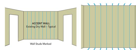
• Using a chalk line stretched between bottom and top mark, snap a line. Use painters tape at top & bottom of **each** stud on floor and ceiling to identify nailing points.
