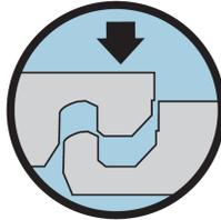
THIS PRODUCT HAS A UNIQUE FOLD-DOWN END JOINT LOCKING SYSTEM! A VINYL SEAM-ROLLER OR WHITE RUBBER Mallet IS RECOMMENDED TO ACHIEVE A FLAT, EVEN SEAM. To avoid installation damage: Do not use excessive force to engage the locking mechanism!
