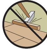
NEVER USE A TAPPING BLOCK OR TOOLS DESIGNED FOR OTHER TYPES OF LAMINATE FLOORS. USING THESE TOOLS MAY DAMAGE YOUR FLOOR AND WILL VOID YOUR WARRANTY
