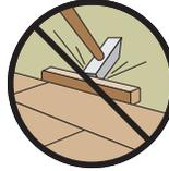
NEVER USE A TAPPING BLOCK OR TOOLS DESIGNED FOR OTHER TYPES OF LAMINATE FLOORS. USING THESE TOOLS MAY DAMAGE YOUR FLOOR AND WILL VOID YOUR WARRANTY
