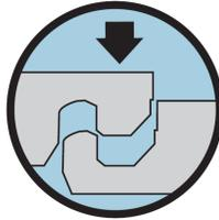
THIS PRODUCT HAS A UNIQUE FOLD-DOWN END JOINT LOCKING SYSTEM! A VINYL SEAM-ROLLER OR WHITE RUBBER Mallet RECOMMENDED TO ACHIEVE A FLAT, EVEN SEAM. To avoid installation damage: Do not use excessive force to engage the locking mechanism!
