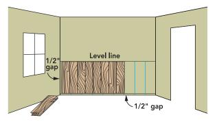
• The last row will need to be cut lengthwise to fit properly, leaving a 1/2" for expansion.
