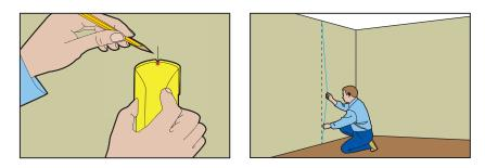
• Using a stud finder to identify studs, mark top and bottom of studs using a pencil.
